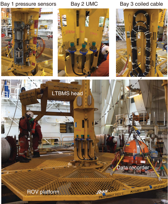
Figure F15. LTBMS head, showing configuration of each bay (top) and ROV platform and data recorder (bottom). UMC = underwater mateable connectors.
