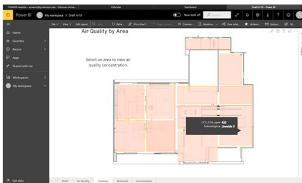
Fig. 7. PowerBI based visualization of interpolated distribution of air quality throughout laboratory space
