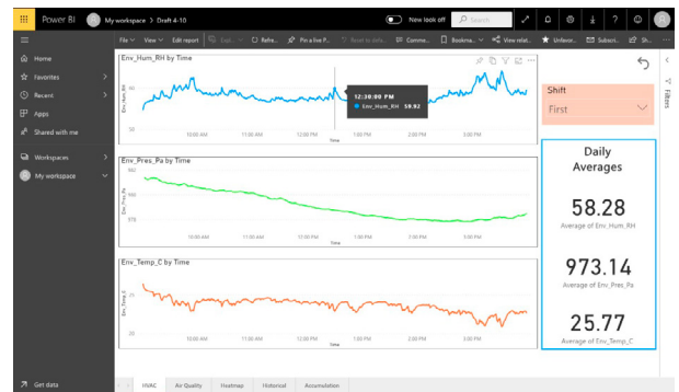
Fig. 5. PowerBI based visualization of temperature, pressure, and humidity for one sensor output. Full page figure available in Appendix B
