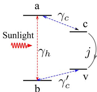
**Fig. 1** Scheme of a donor-acceptor/solar-cell model. The red lines show the coupling to the hot bath, while blue lines show the coupling to the cold bath. The output is denoted as an arc, and the incident sunlight is marked as a wavy line
