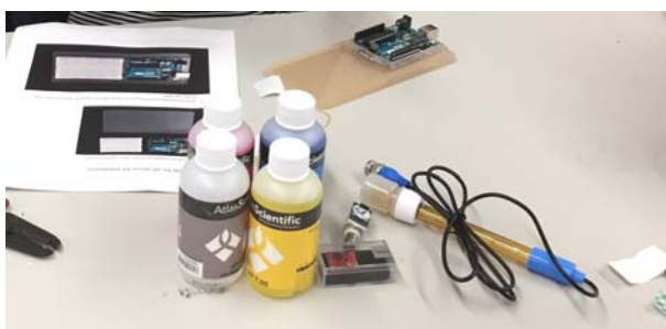
Figure 2. Materials from Arduino and Atlas Scientific that were used to build and calibrate the pH sensor.
