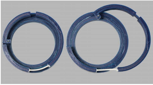
Fig. 3 A 3D printed prototype of the expanding cylinder mechanism with one initially curved flexure, highlighted in white. The shape of the deflected flexure suggests it is loaded with end forces and moments, similar to a traditional fixed-guided beam.
