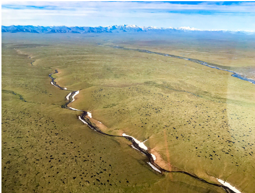
FIG. 9. Thermokarst pits in undisturbed terrain of the 1002 Area of the Arctic National Wildlife Refuge, east of the Jago River. The numerous small thermokarst ponds (up to ~5 m diameter) are caused by thawing of the upper surface of ice wedges that separate the ice-wedge polygons. Thermokarst such as this has recently become widespread across large areas of undisturbed tundra in northern Alaska, and is now common on upland surfaces of the 1002 Area (Jorgenson et al. 2018) (photo: M. Nolan).
