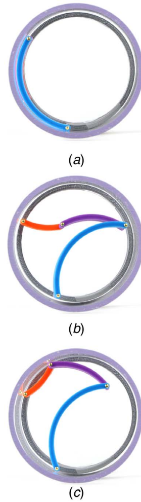
Fig. 16 A Class 3 intramobile mechanism moving from: (a) conformed crossed position, (b) the toggle position, and (c) reaching the limit of intramobile motion, where the short grounded link has rotated \delta_{intramobile,max} (Condition 1)
