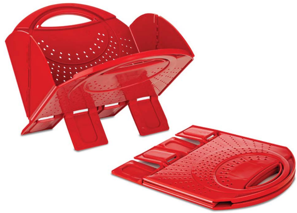
Fig. 7 An origami-based colander that uses the limited facet extension technique in combination with the loading condition (gravity) to achieve stability in its unfolded state (image used with permission from B&R Plastics, Inc ® )
