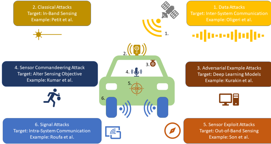
Fig. 1: Examples of different attacks on an autonomous vehicles as classified by our lexicon. 1 refers to the GPS Data Spoofing attack as described by Oligeri et al. 2 is the Classical Spoofing/Jamming attack on lidar as conducted by Petit et al. against lidar. 3 represents Algorithmic attacks generated by Kurakin et al. for deep learning image classification. For 4, we select the Sensor Commandeering Sleuthing attack by Kumar et al. against in-car Automatic Speech Recognition (ASR). In 5, we show the Sensor Exploit Spoofing attack against gyroscopes by Son et al. Finally, 6 refers to the Signal Sleuthing/Spoofing attack completed by Roufa et al. against tire pressure networks.
