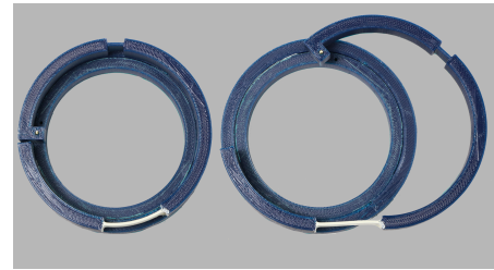
FIGURE 3. A 3D printed prototype of the expanding cylinder mechanism with one initially curved flexure, highlighted in white. The shape of the deflected flexure suggests it is loaded with end forces and moments, similar to a traditional fixed-guided beam.
