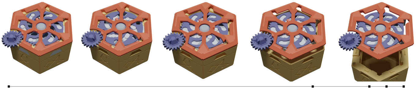
Fig. 1. Expanding Lock Box. An intricate locking mechanism designed for 3D printing can be directly simulated with our algorithm. As the “key” turns, the central spiral is rotated which in turn pulls in each of the five locking pins. When all pins have been retracted the bottom is able to freely fall. Our algorithm’s intersection-free guarantee enables the automatic testing of designs without the need to tune simulation parameters. ©Angus Deveson.
