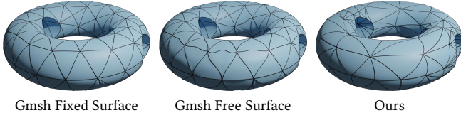
Fig. 22. Example of a BRep meshed with Gmsh where the optimization fails to untangle elements when fixing the surface. By allowing the surface to be modified, the mesh becomes “wiggly”. Our method successfully generates a positive curved mesh.
