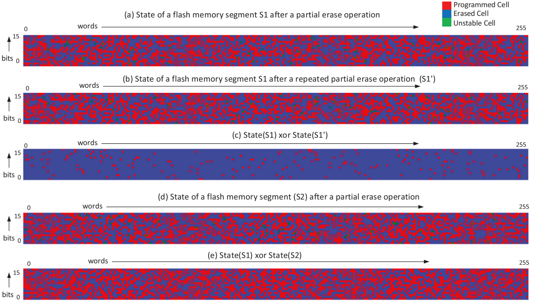
Fig. 9. State of partially erased flash segments.
