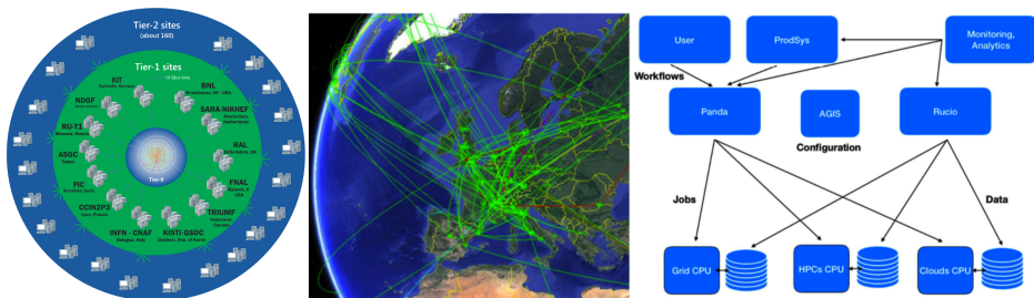
Figure 1: At left: the WLCG infrastructure which, across its Tier0, Tier1, and Tier2 centers, provided the bulk of the computing capacity for LHC Run 1 and Run 2 processing, storage, simulation and analysis. At right, distributed computing system components (in this case ATLAS [3]) which are typical of the LHC experiments.
