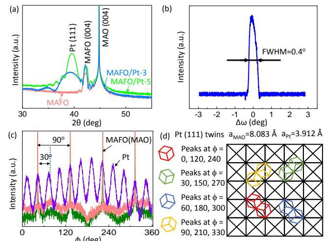
FIG. 1. XRD analysis of samples. (a) XRD  $2\theta/\omega$  scans of MAFO (13 nm)/Pt (5 nm), MAFO (13 nm)/Pt (3 nm), and MAFO (13 nm). (b) Rocking curve scan about the Pt (111) peak for the MAFO (13 nm)/Pt (5 nm) sample shown in (a), with  $FWHM \approx 0.4^\circ$ . (c) XRD  $\phi$  scans on the (113) plane of the MAFO (13 nm)/Pt (5 nm) sample. Pink: MAFO. Green: MAO. (d) Lattice matching relationship between the Pt and MAFO (MAO) unit cells.
