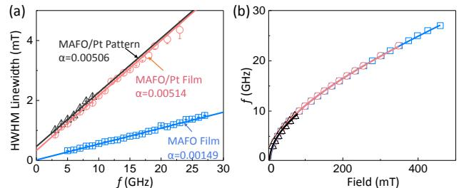
FIG. 6. Frequency dependence of (a) linewidth and (b) resonance field a bare MAFO film (13 nm), unpatterned MAFO (13 nm)/Pt (5 nm) film, and patterned MAFO (13 nm)/Pt (5 nm) ST-FMR strip.
