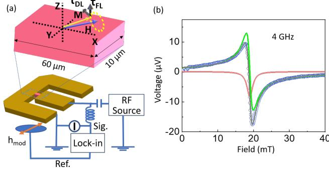
FIG. 2. ST-FMR measurement setup. (a) MAFO/Pt stack etched to a \$60\text{ }\mu\text{m} \times 10\text{ }\mu\text{m}\$ strip. Magnetization, external field, rf field, and SOTs are shown as the arrows. The ground-signal-ground Au electrode connects MAFO/Pt to the external circuit. (b) FMR spectrum at 4 GHz. Red curve: symmetric Lorentzian contribution. Green curve: antisymmetric Lorentzian contribution. blue curve: total fit.
