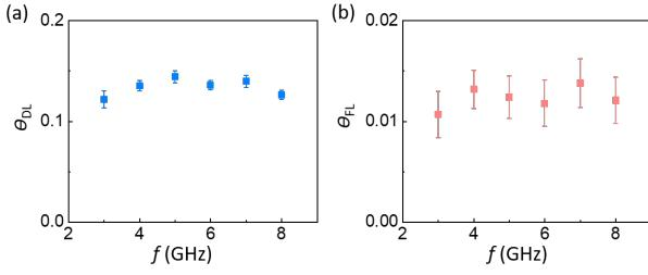
FIG. 8. Dependence of SOTs in MAFO (13 nm)/ Pt (5 nm). (a) Damping-like torque efficiency  $\theta_{DL}$ . (b) Field-like torque efficiency  $\theta_{FL}$ .
