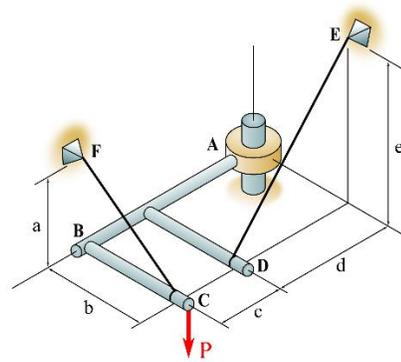
1. Draw the appropriate Free Body Diagram required that will allow you to solve for the forces in the cables.
