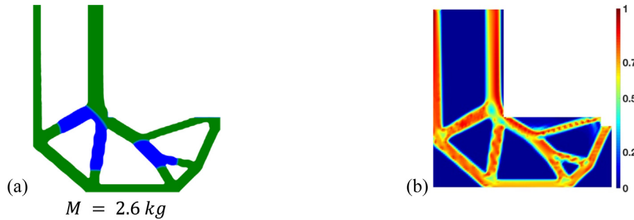
Fig. 15. L-bracket optimization results with failure and relaxed compliance constraints: (a) topology and material distribution; (b) normalized von Mises stress.
