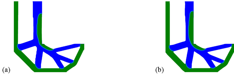
Fig. 14. L-bracket optimization results with failure and compliance constraints with two levels of mesh refinement: (a) 12,800 elements; (b) 25,600 elements.
