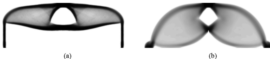
Fig. 15. Optimized (a) stress-constrained and (b) compliance-based designs.
