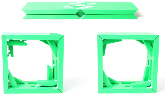
Figure 31. Flat-foldable square unit cell in flat, deployed, and locked states.
