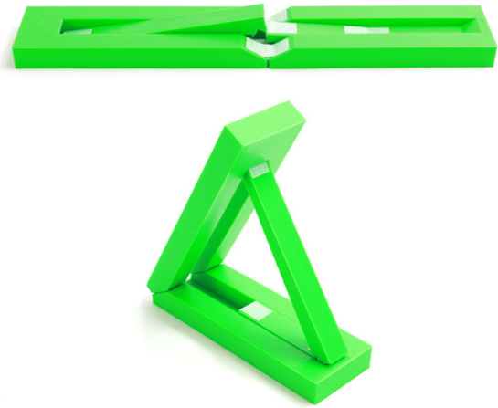
Figure 4. Planar deploying strut ThUDS with arbitrary joint offsets. Shown in flat and deployed states.
