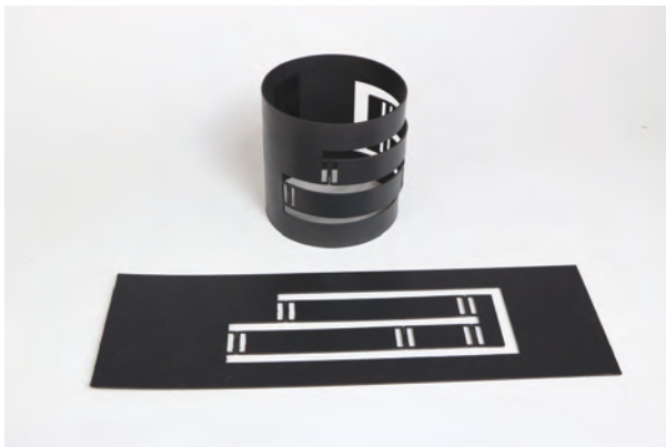
FIGURE 8: A polypropylene cylindrical developable mechanism in its flat and formed states. The pattern was cut with a laser cutter and formed with a cylindrical mold.
