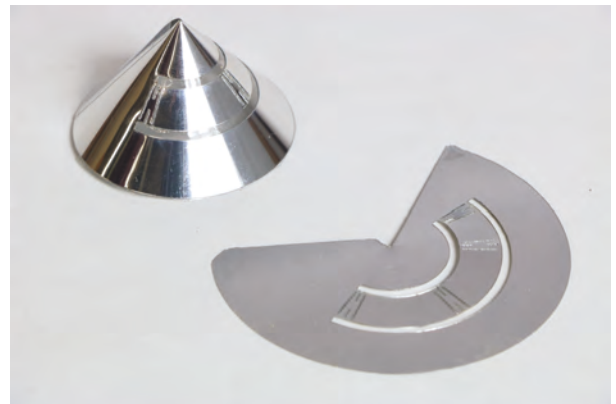
FIGURE 10: A conical developable mechanism made from PET. The pattern was cut on a laser cutter and formed by heat setting.
