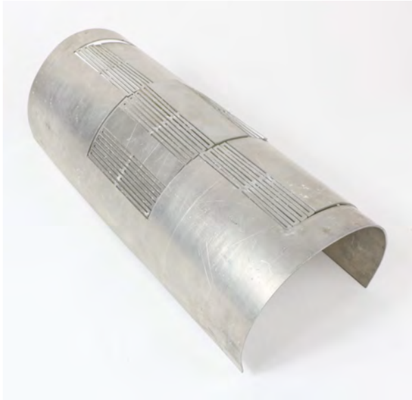
FIGURE 7: The flat pattern of a cylindrical developable mechanism was cut with a water jet in aluminum and formed with a slip roll [39]. During the forming process, the mechanism was attached to a sacrificial layer to ensure the links and surface had the same curvature.
