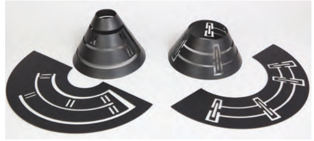
FIGURE 9: Various polypropylene conical developable mechanisms in their flat and formed states. The two dimensional patterns were cut with a laser cutter, and formed in a conical mold.
