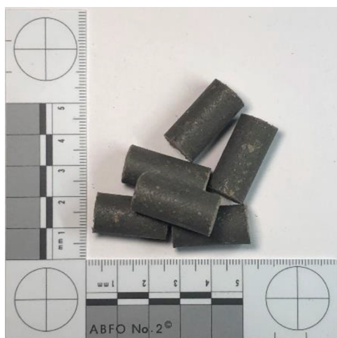
Figure 12. Pellets produced from fiber–plastic mix waste (60:40 ratio) of \phi 12.7 mm diameter and 25.4 mm length.
