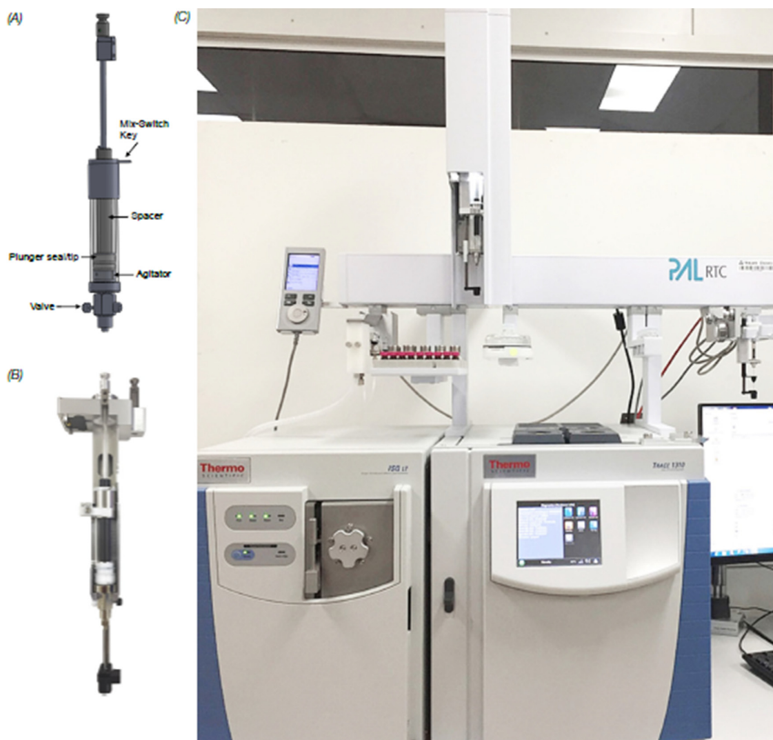
Fig. 6. Fully automated micro-LLE system. (a) the current version of a micro-LLE syringe, (B) the current version of the micro-LLE syringe on a PAL tool, and (C) the automated micro-LLE system. Copyright (2021) Trajan Scientific and Medical Technical Poster (Part #: TP-0236-G) [Ref. 103].
