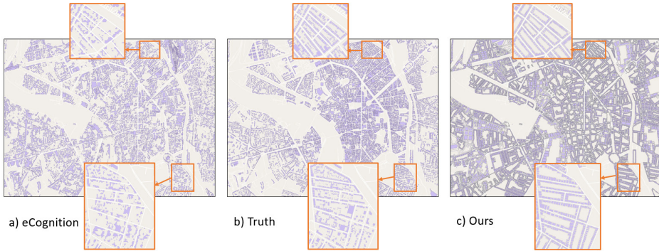
Fig. 11. Segmentation Comparison Images. We compare the results of our approach to directly extruding the segmented and labelled satellite image provided as input. a) Segmentation and labeling result of using eCognition. b) Ground truth segmentation and labeling. c) Our produced procedural model with labeling.
