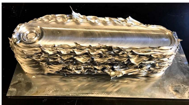
Fig. 18 Multilayer deposit of AA2219 developed by the AFSD technique [147] (Reprinted with permission from Elsevier © 2021)
