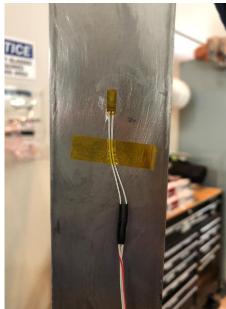
Figure 3: Strain gauge installed on one side of the beam
