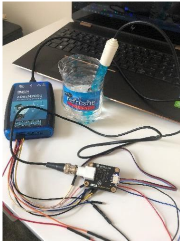
3a. pH sensor with M1K device
