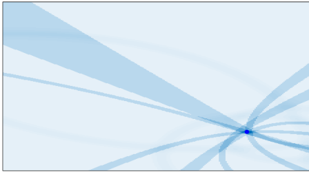
Figure 7: OwLL uses particle filtering atop the measured TDOA hyperbolas to estimate the location of the client
