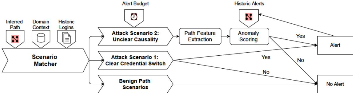
**Figure 4:** Architecture of Hopper’s alert generator (§ 6). Given a login path (§ 5), Hopper checks whether the path matches a benign scenario or an attack scenario. Based on the path’s scenario, Hopper either discards the path or generates an alert if the scenario’s detector triggers.
