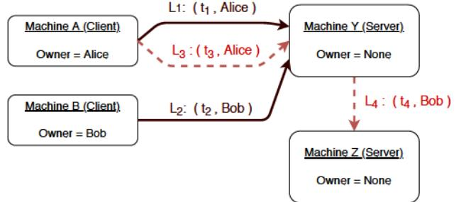
**Figure 3:** An example of a simple login graph. Solid black edges ( $L_1$  and  $L_2$ ) correspond to benign login events. Dashed red edges ( $L_3$  and  $L_4$ ) correspond to a lateral movement attack path.
