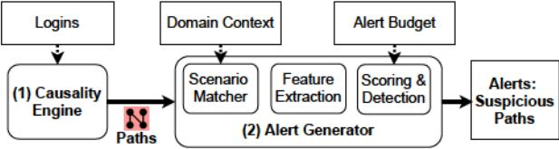
**Figure 2:** Hopper analyzes login events between internal machines within an enterprise and generates alerts for paths of logins that correspond to suspicious lateral movement activity. Hopper has two key components: (1) a causality engine that infers a set of causal paths that a login might belong to (§ 5), and (2) detection and scoring algorithms that decide whether to alert on a path of logins (§ 6).
