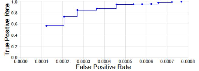
**Figure 5:** ROC Curve for Hopper’s unclear causality detector (§ 6.2) at different budgets (1–11 daily alerts). The True Positive Rate reports the fraction of (180) attacks with unclear causality that Hopper detects. The FP Rate reports the number of false alarms divided by the number of logins in our evaluation data (2.94M).
