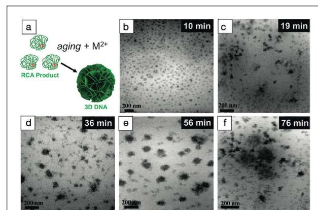
**Figure 3.** Liquid phase scanning transmission electron microscopy observation of the nanostructure assembly from functional nucleic acids; formation of spherical nuclei, growth and agglomeration of crystallites, and nanoflower assembly.<sup>29</sup>
