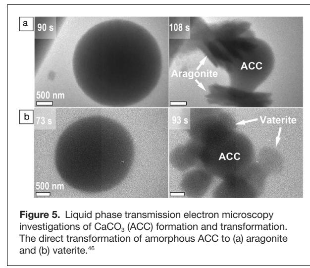
**Figure 5.** Liquid phase transmission electron microscopy investigations of  $\text{CaCO}_3$  (ACC) formation and transformation. The direct transformation of amorphous ACC to (a) aragonite and (b) vaterite.<sup>46</sup>
