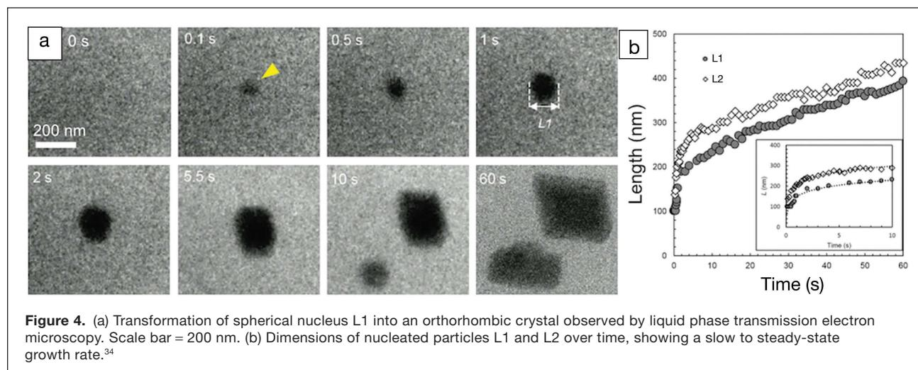
**Figure 4.** (a) Transformation of spherical nucleus L1 into an orthorhombic crystal observed by liquid phase transmission electron microscopy. Scale bar = 200 nm. (b) Dimensions of nucleated particles L1 and L2 over time, showing a slow to steady-state growth rate.<sup>34</sup>
