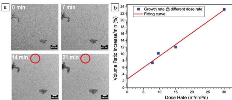
**Figure 8.** Liquid phase scanning transmission electron microscopy studies of CoCO<sub>3</sub> formation and growth. (a) Bright-field scanning transmission electron microscope images of CoCO<sub>3</sub> growth at an electron dose rate of 15.6 e<sup>-</sup>/nm<sup>2</sup>/s. The red circle marks nucleation of a new primary particle. (b) Linear dependence of the volumetric growth rate of amorphous CoCO<sub>3</sub> particles on electron dose rate.<sup>42</sup>
