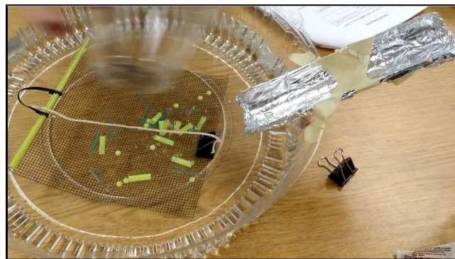
Figure 2 - A photo of a floating filter and a screenshot of a video of the filter test
