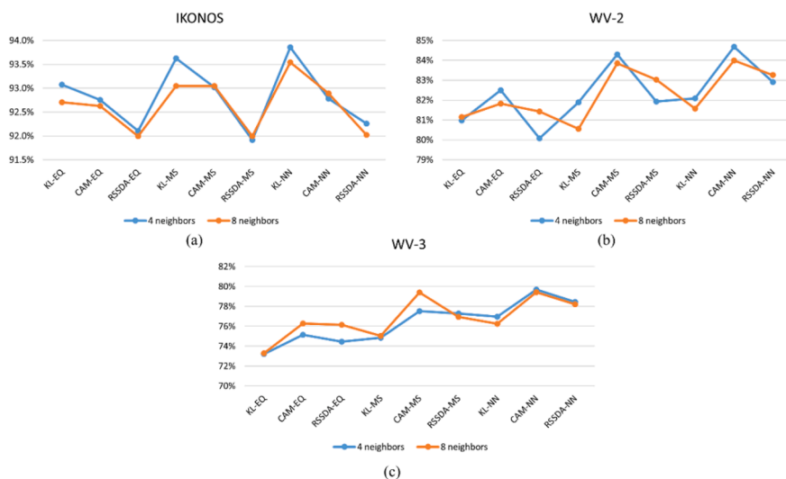
Fig. 11. The changes of classification accuracy with the spatial association detected along four and eight directions for nine RCCM methods: (a) IKONOS image, (b) WV-2 image, and (c) WV-3 image.
