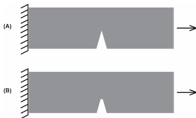
Figure 6. Theoretical examples of crack tips. (A) A sharp crack tip promotes rapid propagation of the crack. (B) A blunt crack tip slows the propagation of the crack.
