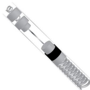
Figure 2. Simplified cross-section of an implantable cardioverter-defibrillator lead.
