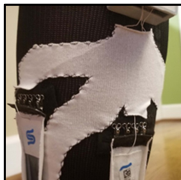
Figure 11. Hook and eye attachment to hold SRS in place.
