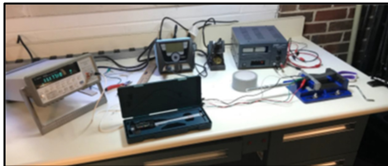
Figure 3. Micro-ohm meter testing setup (Iteration I).
