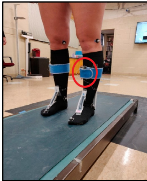
Figure 9. A sock prototype was used for the slip and trip experiment. SRS module location in the red circle.
