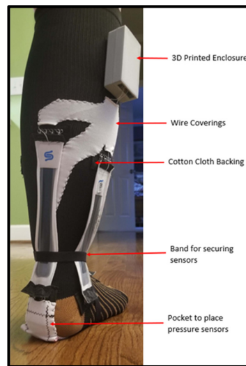
Figure 12. Sock prototype featuring wire coverings and band to form-fit SRS.
