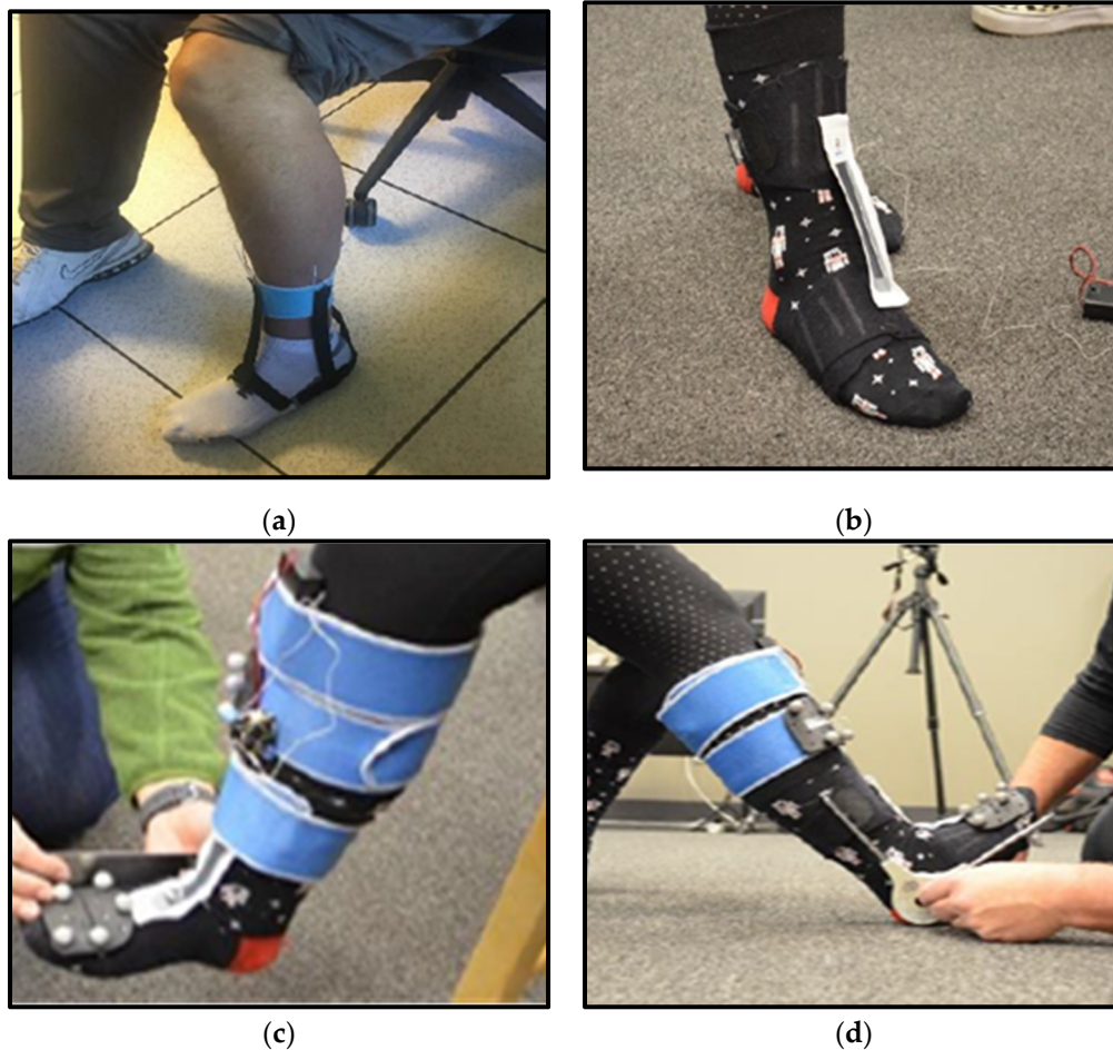
Figure 8. Early attempts at using Velcro to attach sensors to the sock. (a) The initial attempt at mounting SRS with Velcro, (b) SRS mounting SRS to ankle straps with Velcro on SRS only, (c) SRS mounted with motion capture clusters and sensing module, and (d) SRS mounted while the foot is being calibrated to the neutral position.
