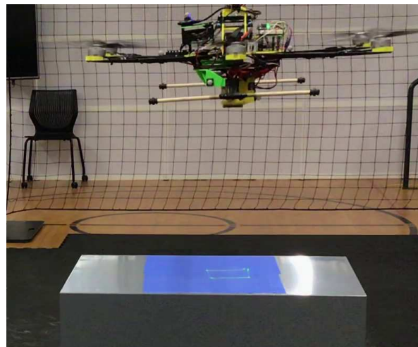
Fig. 1. The 3D printing hexacopter just finished printing a square contour on top of a gray box. A video of this print test can be found at https://youtu.be/tEooDpE2TyE .
