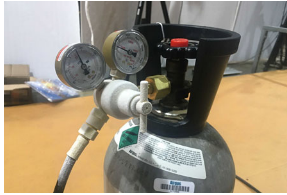
Fig. 2. The regulator and flowmeter mounted on a gas cylinder.
