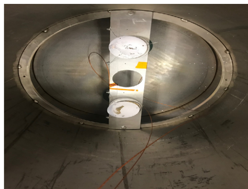
Fig. 4. PMTs mounted with TPB coated acrylic disks inside IV after an initial test fill. A ring of TPB can be seen on the bottom side of the IV above the welded steel ring. Small TPB particulate can be seen on the bottom of the IV.
