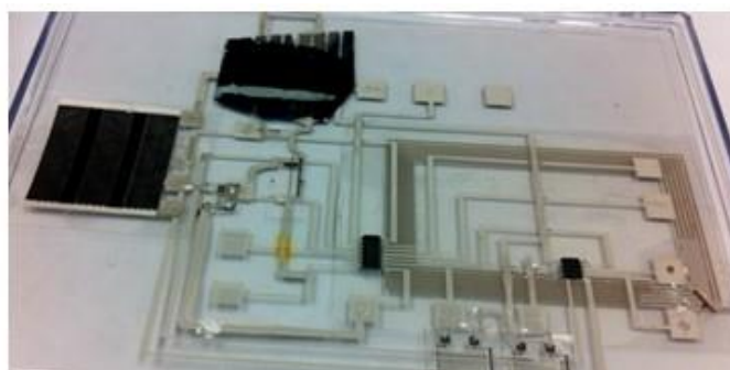
Figure 2. Printed light and temperature wireless sensor, as an example of hybrid flexible electronics, with some printed TFT circuits, some conventional components and printed silver interconnects. (Ref. 9; Schwartz et al)
