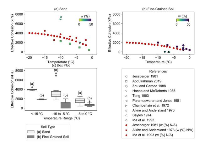
554 Figure 13. Variations of effective cohesion with temperature for (a) sand and (b) fine-grained
