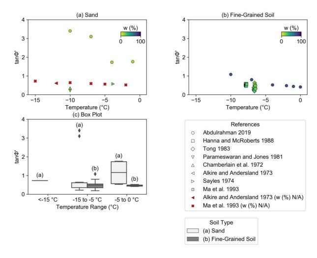
549 Figure 12. Variations of the tangent of effective friction angle with temperature for (a) sand and
