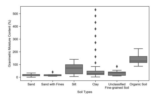
*331* Figure 4. Box plots of gravimetric moisture content for various types of permafrost-affected *332* soils. Sample size of gravimetric moisture content is 184 (outliers are shown as rhombus *333* markers).
