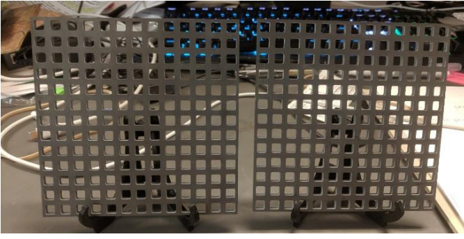
Fig. 7. Fabricated perforated lossy magneto-dielectric (MF500F-112).
