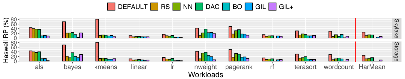
Figure 7: Relative performance (RP) of each method in mod2high setting when Haswell is the target hardware (lower is better).
