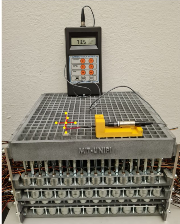
Figure 11. Preliminary measurements of the magnetic field in air (about 10 mm above the magnet) with a portable Gauss-meter F.W. Bell/4048 equipped with a Hall sensor.
