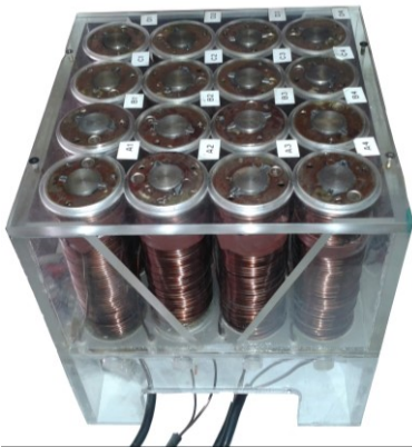
Figure 2. HBB-I prototype and excitation system: the current produced by the four-by-four array of solenoids produces the magnetic field [12].
