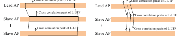
Fig. 6: Extracting the signal frame for one STA at the AP processor via correlating signal streams with L-LTF.
