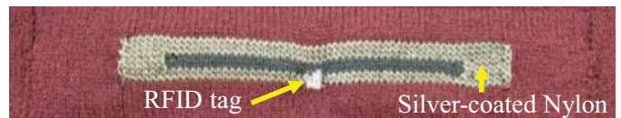
Fig. 1: Bellyband antenna [6]. The conductive part of the antenna is made from silver-coated nylon.
