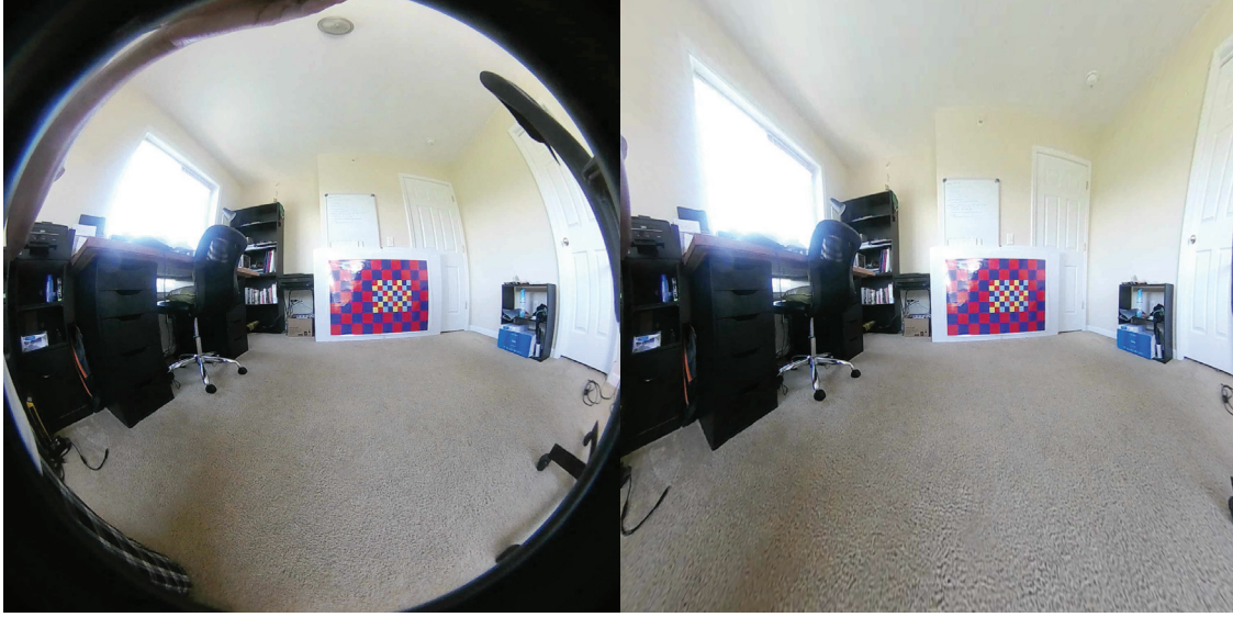
Fig. 4 Original omnidirectional camera image (left) and undistorted omnidirectional camera image (right)
