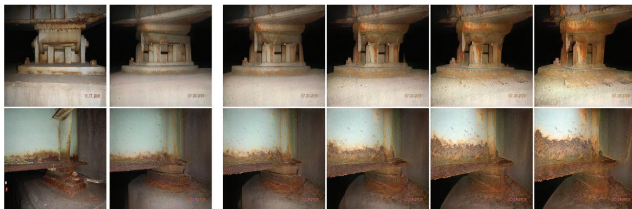
Figure 1. Examples of semantic deterioration forecasting. Where the first image on the left is the real image and the following image is the embedded version of that image. The subsequent sequence of images are increments towards the target corrosion boundary by a relative gain of (3.0, 4.0, 5.0, and 6.0) respectively.
