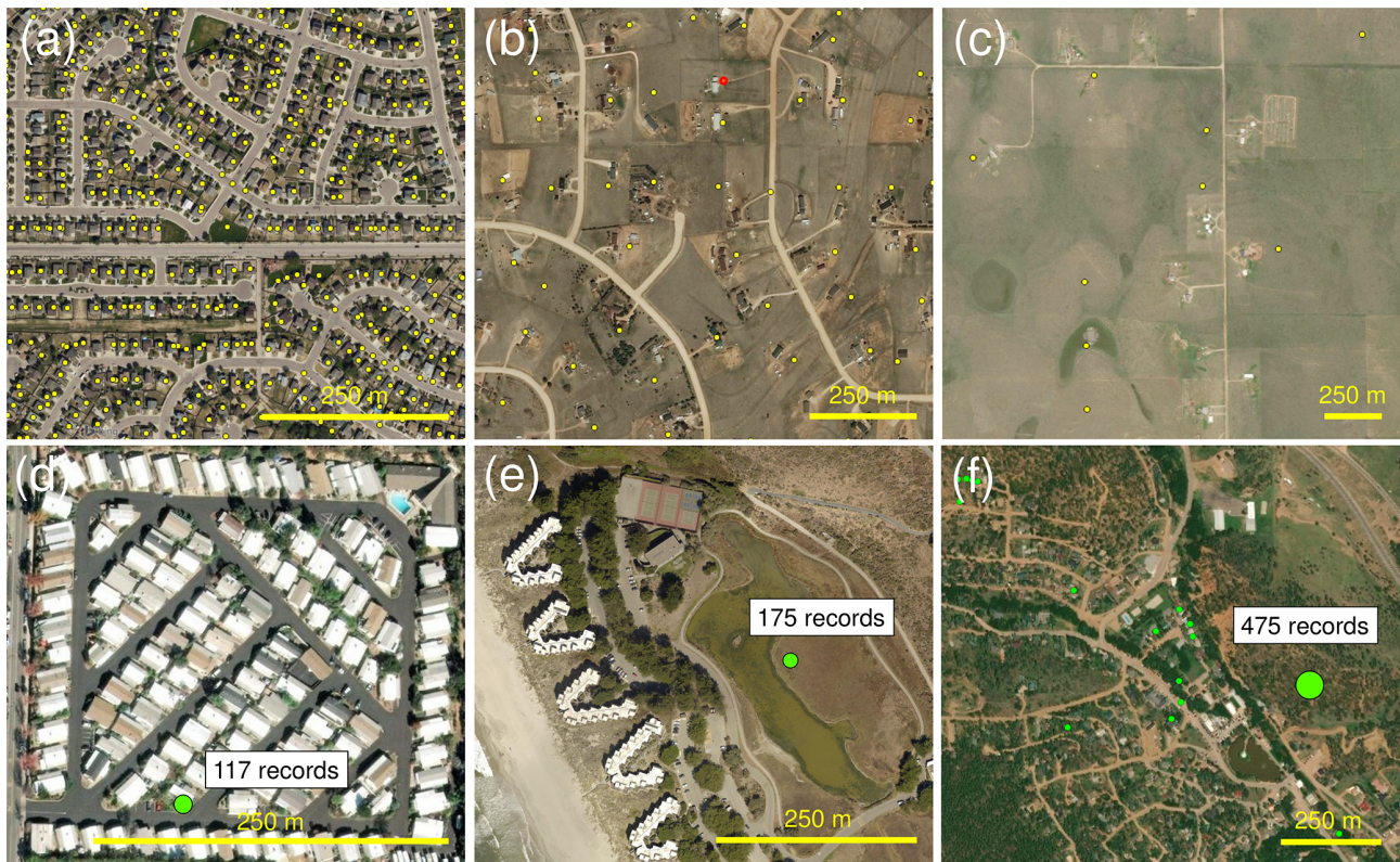
Figure 7. Variations in positional accuracy and generalization levels in the ZTRAX database: example of (a) highly accurate settlement locations in a dense residential neighbourhood dominated by single-family homes, (b) settlement locations of medium positional accuracy, and (c) settlement locations of low positional accuracy in rural parts of the USA. Spatially generalized settlement locations (i.e. multi-record locations) for (d) a mobile home park and (e) a planned community or condominium; (f) a rare agglomeration of records, likely resulting from pseudo-locations assigned during database work in progress. Base map imagery from © Microsoft 2020.
