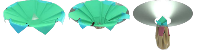
Fig. 7. Funnel. Three cloth panels ( \mu = 0.4 , 26K nodes each, strain upper bound at 1.0608) are dropped on a funnel. Under friction they rest stably on top until a sharp, scripted collision object rapidly pulls the panels down.
