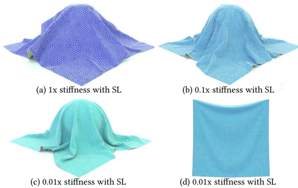
Fig. 13. Anisotropic strain limiting. We apply the C-IPC anisotropic strain-limiting model to the sphere drape test in (a) through (c), varying only scaling of the measured membrane stiffnesses, and to the two-corner cloth hang test in (d). All are time stepped at h = 0.04s with their final equilibria shown here. In (c) and (d), with a 0.01\times scaling of the measured stiffness, we see that C-IPC’s tight enforcement of the measured strain limits [Clyde 2017] obtains artifact-free drapes with differing wrinkle patterns resulting from the anisotropic model.
