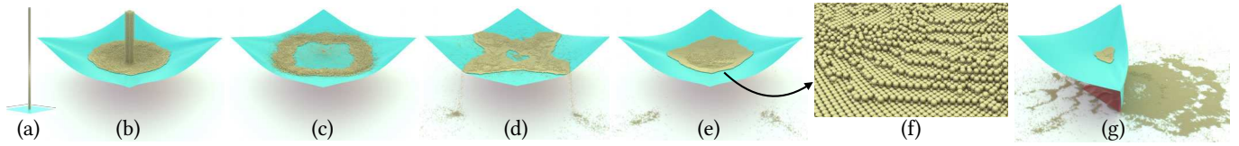
Fig. 22. Granules on cloth. We drop a column of 50K particles onto a cloth with fixed corners. Each particle is represented by a single node, with C-IPC offset and \hat{d} set to 2mm and 1mm respectively in order to capture the granule’s volume at rest while the C-IPC barrier ensures particles do not tunnel through each other nor the cloth shell. Particles at rest capture tight spherical packings (see zoom in) confirming offsets are preserved throughout. Finally we release one corner of the cloth to let the granules fall onto the ground.
