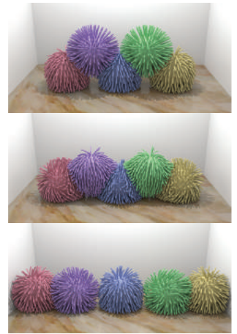
Fig. 15. When we push medial IPC to simulate five puffer balls, the subspace size is almost 100K. In this case, we choose CPU for system solve. In this extreme reduced simulation, medial IPC is 14 \times faster.
