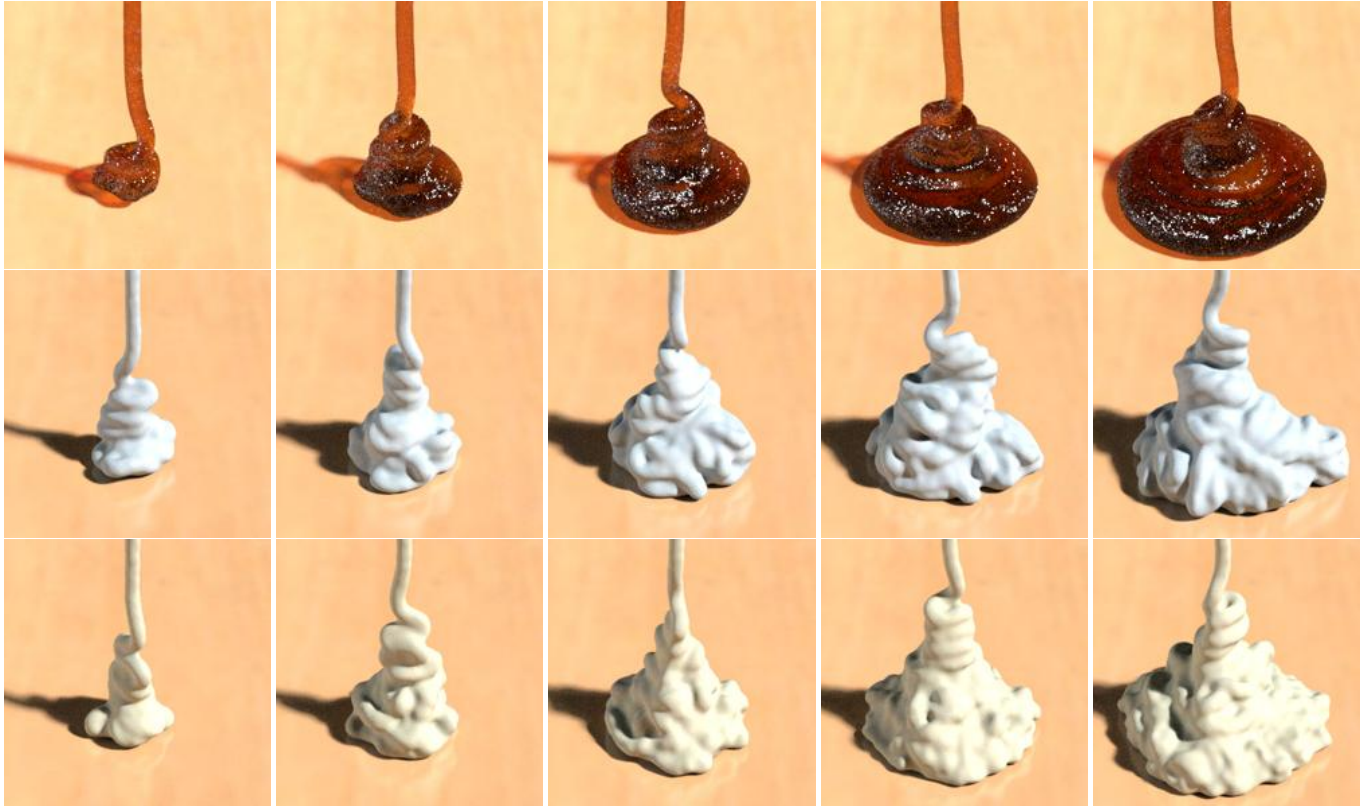
Fig. 2. Our unified constitutive model can generate the classical liquid rope coiling effect (top) for Newtonian viscosity [Larionov et al. 2017], and also asymmetric coiling and elastic effects for non-Newtonian liquids (middle and bottom) such as Oldroyd-B [Ram et al. 2015] and Pom-Pom [Bishko et al. 1997]. A columnar structure is first generated by high-frequency coiling, which collapses at a certain point and the process repeats - showcasing secondary coiling . The average \Delta t during simulations for each case is \Delta t = 10^{-5} s.
