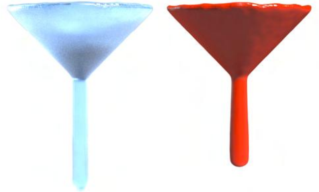
Fig. 13. A closer view of die swell in the shear thinning liquid example from Figure 12. After exiting the throat of hourglass, the shear thinning stream swells (right), while the Newtonian liquid (left) does not. The average \Delta t during simulations is 10^{-5} s.
