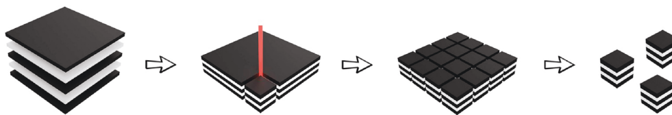
Fig. 6. Schematic of device fabrication by laser cutting.
